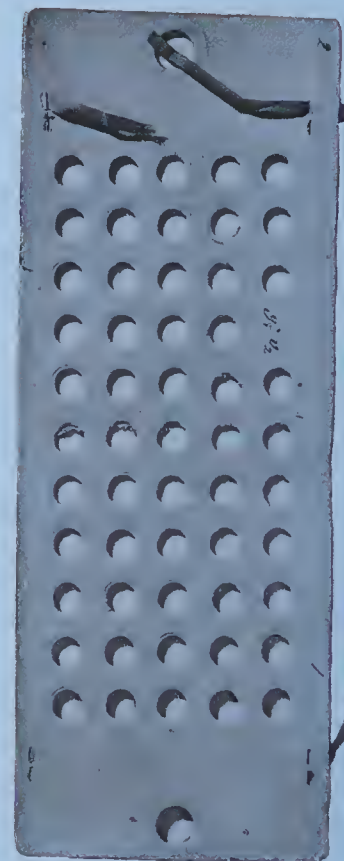
Punch card designed by Babbage for his Analytical Engine.
