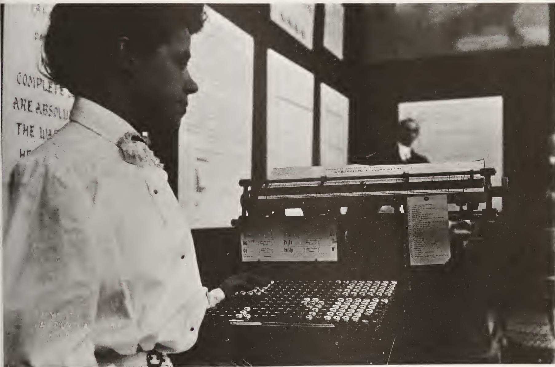
Powers electric card-punching machine. With this machine, the information was keyed in, then punched all at once into the card.
