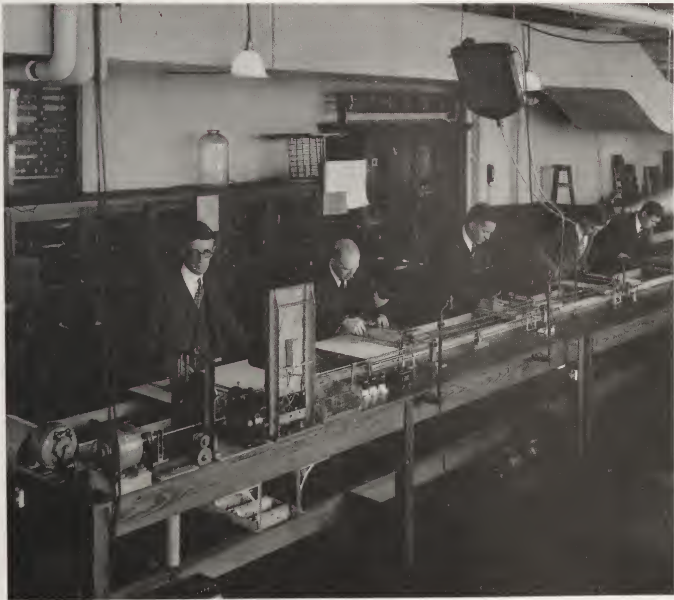
Vannevar Bush with F. G. Kear, H. L. Hazen, H. R. Stewart, and F. D. Gage using the product integrator. The equations to be integrated were plotted by hand on sheets of paper. These were then slowly passed under pointers, and operators stationed along the machine kept the pointers on the curves.
