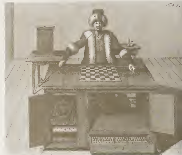
The elaborate gears and compartments in von Kempelen's chess player cleverly concealed the man hidden inside.
