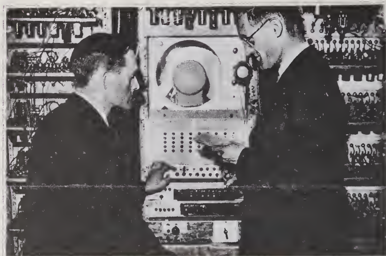
ABOVE: THE CONTROL PANEL OF THE AUTOMATIC SEQUENCE-CONTROLLED CALCULATING MACHINE, AT MANCHESTER UNIVERSITY, SHOWING THE MONITOR CATHODE RAY TUBE WITH DR. T. KILBURN ON LEFT, AND PROFESSOR F. C. WILLIAMS, INVENTOR OF THE MEMORY STORAGE SYSTEM EMPLOYED, ON RIGHT. FEEDING A PROGRAM INTO THE MACHINE. LEFT: ONE OF THE CATHODE-RAY STORAGE TUBES, SHOWING THE POINTS OF LIGHT INDICATING A MATHEMATICAL PROBLEM IS BEING SOLVED.
